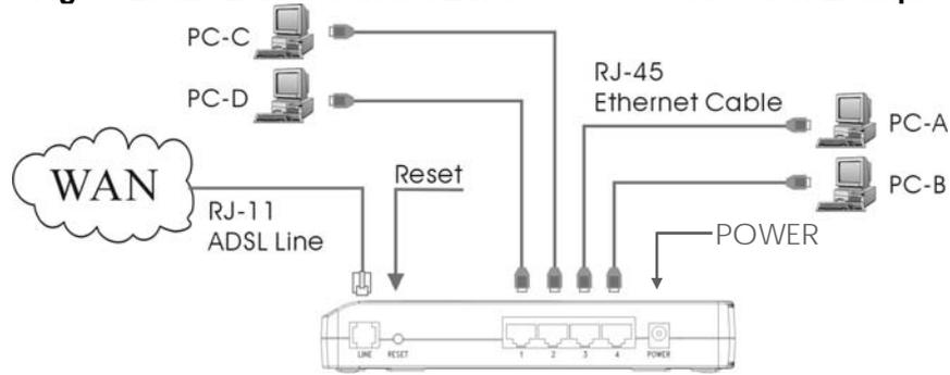
Complete the following steps to connect the cables to the ADSL Router:
