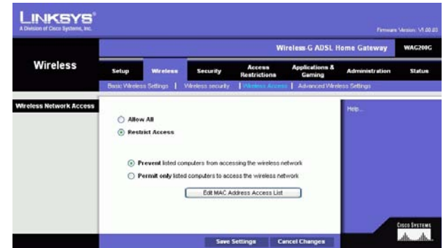
Abbildung 5-17: „Wireless Network Access“ (Wireless-Netzwerkzugriff)
